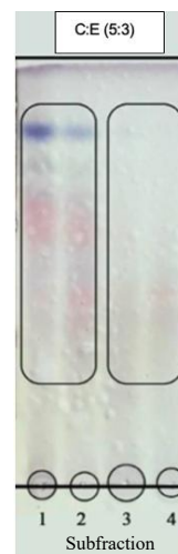
Figure 2. TLC chromatograms of TCM 2 subfractions visualized after spraying with vanillin–sulfuric acid reagent
